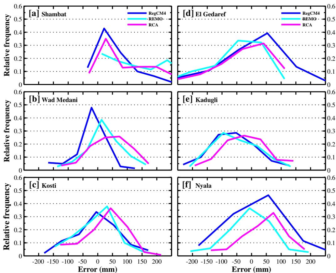
Fig. 9. Probability density function of the error in monthly rain amount computed for April to October. The rest of the year is excluded because it has high likelihood of zero error.
