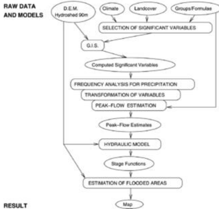
Figure 2 : Scheme illustrating the full workflow to obtain flood hazard maps for different return periods Source: GAR,2011
